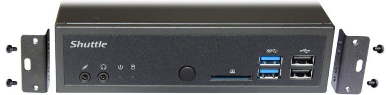
2. Please place the PC behind the opening of the front plate and affix the PC with four screws from the front.
