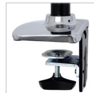
Desk Clamp attaches to surface edge .4" to 2.4" (1 to 6 cm) thick; Grommet Mount attaches through surface holes .31" to 2" (8 to 50 mm) wide and up to 3" (7,6 cm) thick
